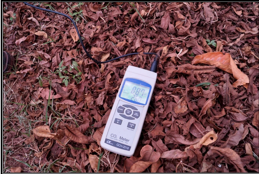
Fig. 10. Abnormally high carbon dioxide level on the litter bed, which may be attributed to the gradual decomposition of the leaf litter by microbial action
